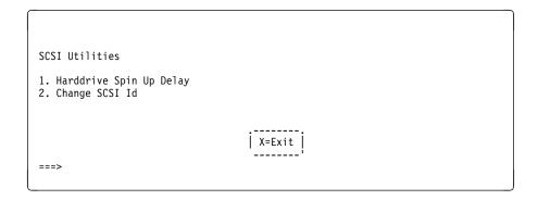
Using the **Harddrive Spin Up Delay** option allows you to change the spin up delay time for SCSI hard disk drives attached to your system. Spin up delay values can be entered manually, or you can use a default setting (two seconds). All values are measured in seconds.
